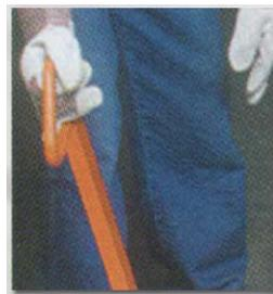
The BLE Series' convenient **BarLift** allows the operator to easily tilt the Leveler rearward, then push it forward onto the truck bed.
